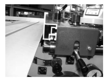
The calibration of the read-out is easy and simple: slide the alu saw fence up against the saw blade so that the teeth just touch the fence, and now push simultaneous both buttons F and SET, now the read-out is set at 0.
