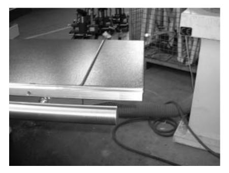
The little table extension as supplied, makes it possible as before to cut upto 1380 mm. It will also act as a protection for the magnetic tape.
